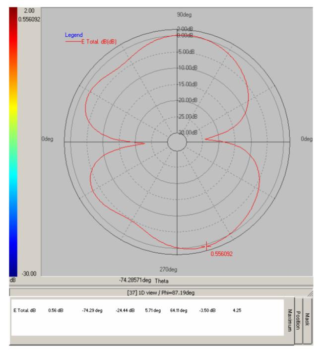
Frequency (MHz): 2450.00Pattern Field: E PlaneAverage Gain: -3.5 dBMaximun Gain: 0.56 dBMaximum Gain (degree): -74.29Minimum Gain: -24.44 dBMinimum Gain (degree): 5.71
