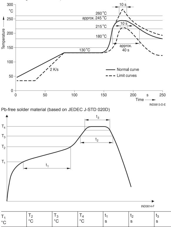
Time from +25 °C to  $T_4$ : max 300 s Maximal numbers of reflow cycles: 3
