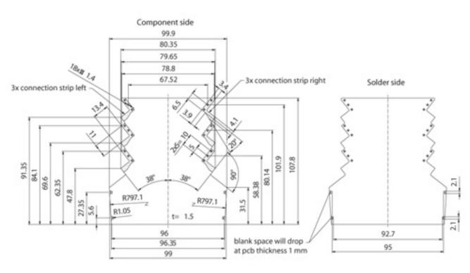
non dimensioned radii max R1 inhibited surface
