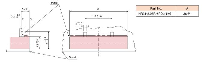
1.2 Recommended mounting panel dimensions (straight through hole type)
