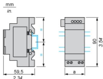
Screw Fixing (Retractable Lugs)
