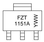
FZT 1151A = Product Type Marking Code YWW = Date Code Marking Y or  $\overline{Y}$  = Last Digit of Year (ex: 5 = 2015) WW or  $\overline{W}W$  = Week Code (01~53)
