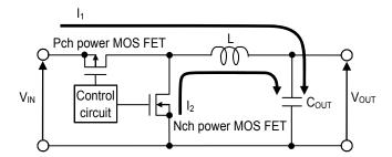
Figure 9 Basic Circuit Drawing of Step-down Switching Regulator
