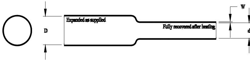
This specification covers the requirements for one type of single wall, electrical insulating, extruded tubing whose diameter will reduce to a predetermined size upon application of heat in excess of 110°C (230°F).
