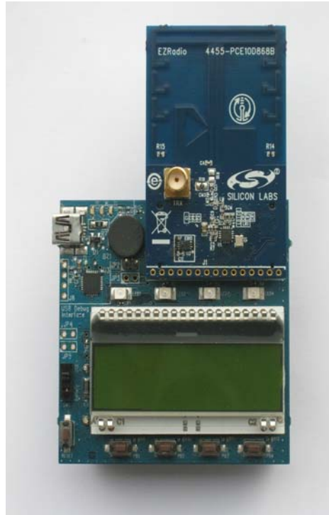
Figure 3. LCD Baseboard with Connected RF Pico Board
