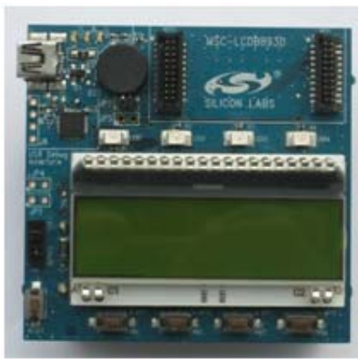
Figure 1. LCD Base Board (P/N MSC-LCDBB930-PER)
