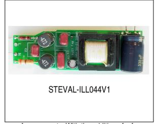
use of components. With the addition of a few extra components the HVLED815PF is made to draw near-sinusoidal input current from the AC line. The circuit regulates LED current over a wide range of line voltage and LED string voltage, and is dimmable with standard Triac-based dimmers.
