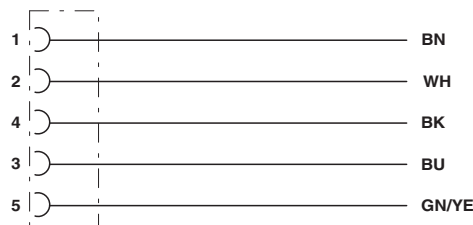
Contact assignment of the M12 sockets
