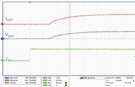
Figure 38. Startup by enable ( I_{OUT} = 300\text{ mA} , normal mode)
