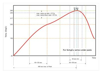
Fig 2. Infrared soldering profile
