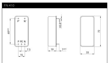
All dimensions in mm; 1 inch = 25.4 mm Tolerances according: ISO 2768-m/EN 22768-m
