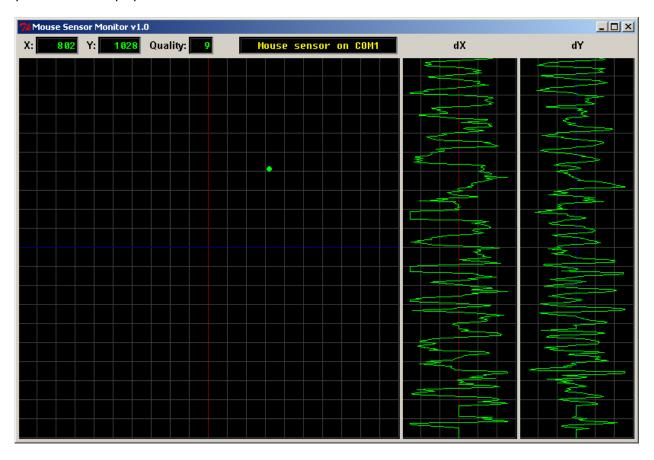
The green dot keeps track of the sensor's current X and Y position. The **dX** and **dY** strip charts track the sensor's instantaneous change in position. If you move the sensor too fast, a message that says "OVERFLOW" will display. The background grid spacing is 250 sensor pixels. The default resolution for the PBASIC program is about 500 d.p.i., which works out to 1/2" of travel per division.
