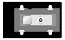
6. (See note below for an alternative to steps 6 and 7.) Place the assembled circuit board over the base assembly, so that the little nibs from the rivets fit into the corner holes of the circuit board. The end of the LED should be very near or just touching the lens assembly:
