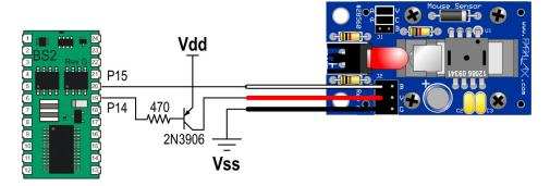
Using this circuit entails a change in the program, since the clock is now inverted from what it was. This is easily accomplished by commenting out the line that says **#DEFINE NEG\_CLK**:
