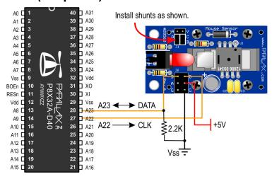
**NOTE:** Do not omit the 2.2K resistor. It is required in order to limit the input voltage to the Propeller.
