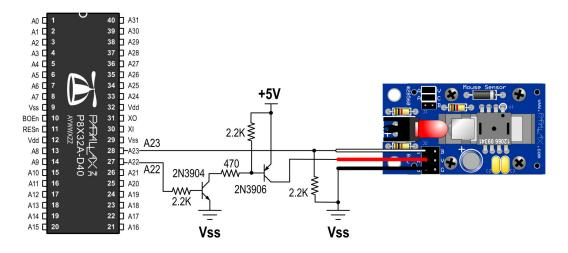
The Spin program requires no changes to accommodate this new circuit. The reason is that the clock signal is inverted twice.
