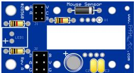
3. Take the LED and insert it into the right-angle holder, being sure to position the longer, positive lead as shown:
