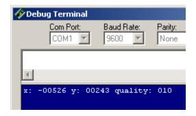
The program accumulates the sensor's X and Y displacement data to show the current position. It also displays a "quality" figure, which indicates how textured the surface is that the sensor is looking at. The higher the number, the better.
