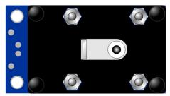
**NOTE:** As an alternative to steps 6 and 7 above, you can first center the spacers over the holes in the base, then position the circuit board on top of these, and simply drop the screws through the holes. The nuts can then be installed from the bottom, one at a time, and the screws tightened.
