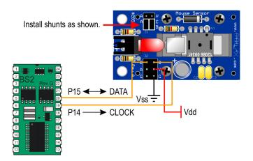
**NOTE:** Board of Education users can simply connect using two extension cables from the onboard servo headers. *Make sure that servo power is jumpered to Vdd and not Vin*.
