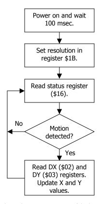
Communication with the chip takes place via two-wire (clock and data) serial I/O. The clock line is normally high and pulses low to transfer data bits in or out of the chip.
