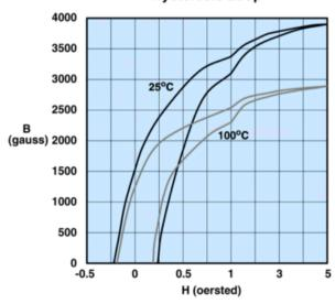
Measured on a 17/10/6mm toroid at 10kHz.
