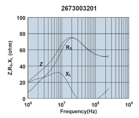
Impedance, reactance, and resistance vs. frequency.
