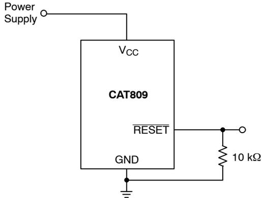
Figure 8. RESET Valid with V<sub>CC</sub> Under 1.0 V
