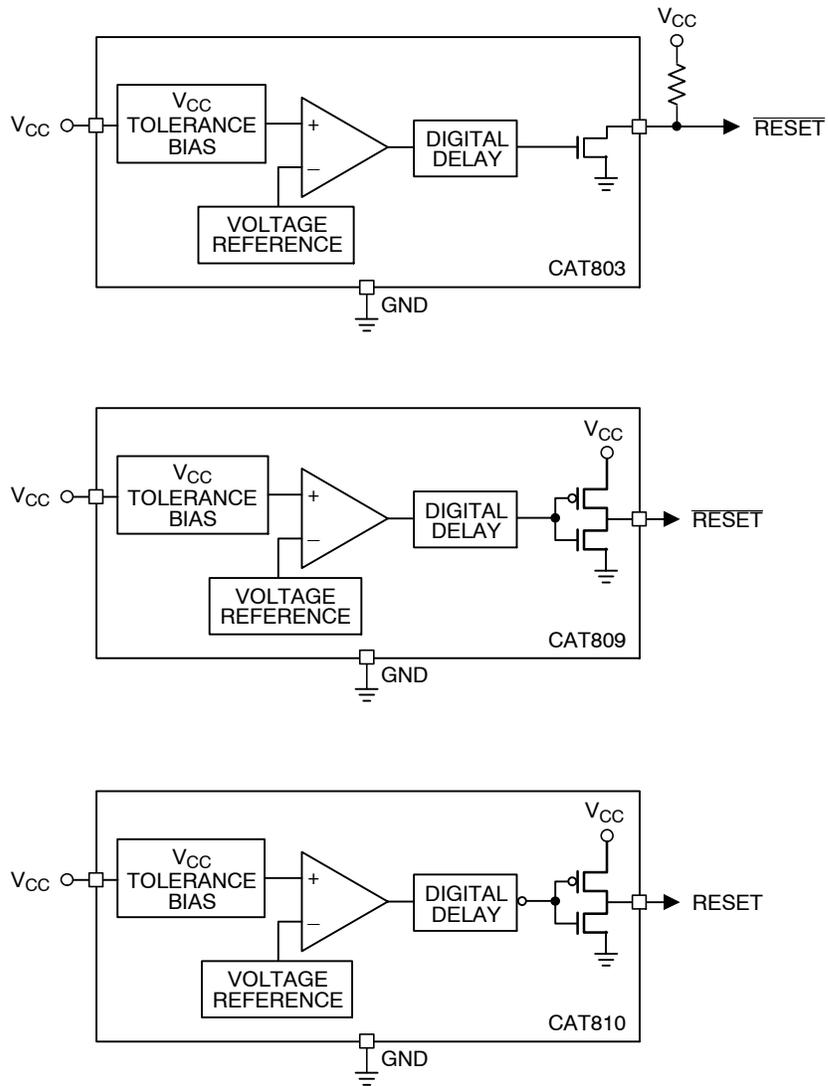
Figure 1. Block Diagrams
