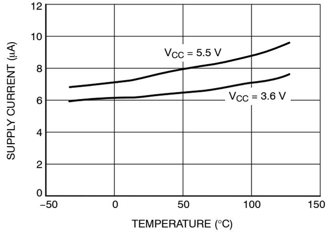
**Figure 3. Supply Current vs. Temperature (No Load, CAT8xxR/S/T/Z)**
