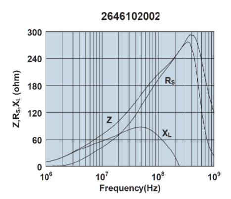
Impedance, reactance, and resistance vs. frequency.
