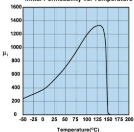
Measured on a 17/10/6mm toroid at 100kHz.
