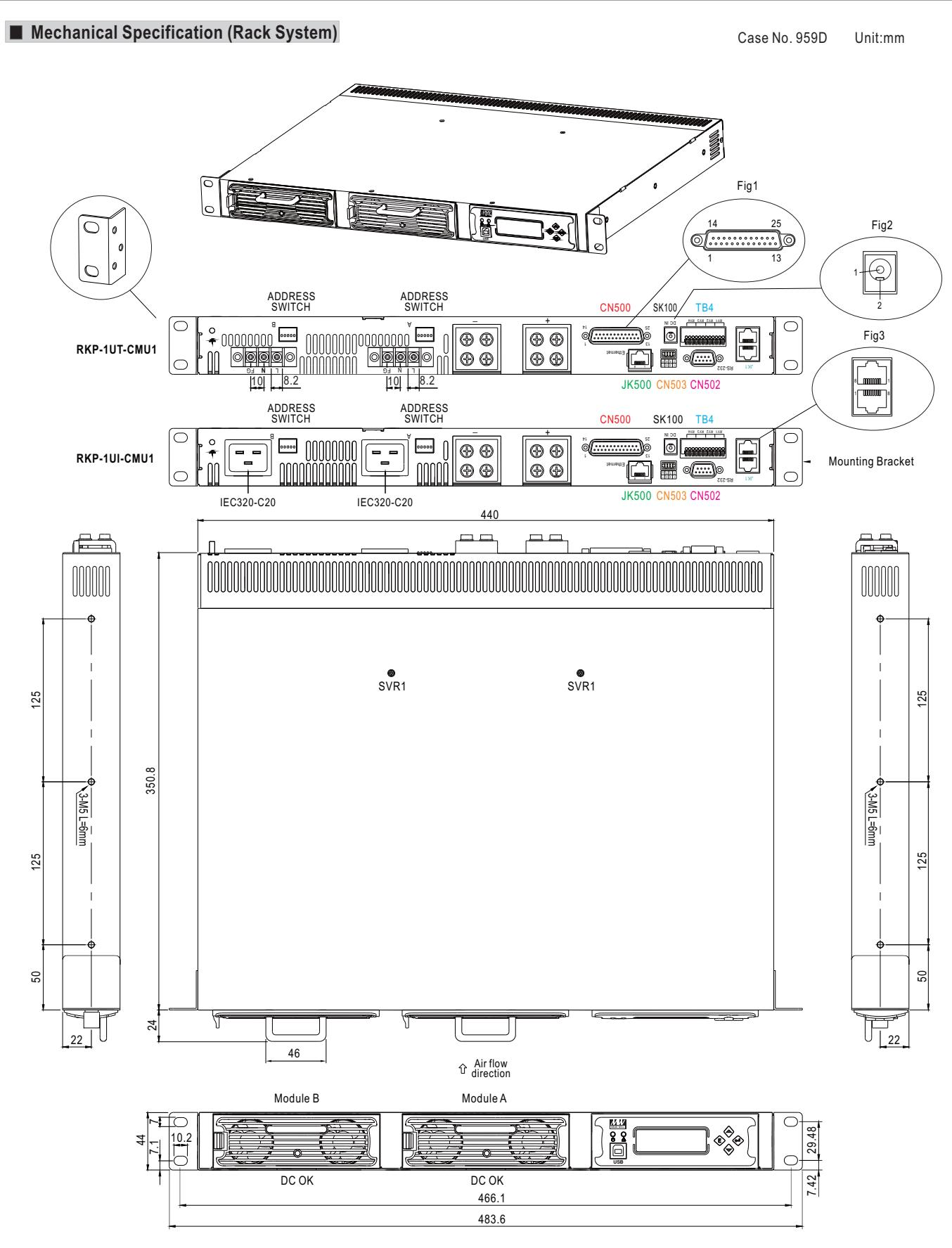
※ IN/OUT Connector Pin No. Assignment([CN500](#)) : D-Type Right Angle 25 positions
