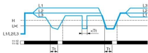
Tt Time delay after crossing of threshold (adjustable on front panel)
