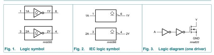
Low-power dual inverter with open-drain output
