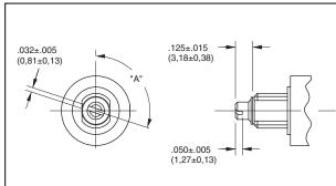
Form, fit and function equivalent to standard shaft switches. The dimensions shown have evolved as the most popular for this type of switch. See Style "B" in the Choices and Limitations chart. Previous users may have ordered these switches by a non-descriptive part number containing a "Y". Contact Grayhill, if in doubt about a cross-reference.
