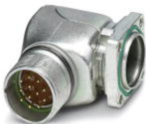
Device connector, front mounting, angled rotatable, Screw locking, M23, number of positions: 17, type of contact: Pin, Crimp connection, Axial O-ring, 4x Ø 3.2, shielded: yes, flange dimensions: 28 mm x 28 mm
