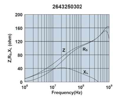
Impedance, reactance, and resistance vs. frequency.
