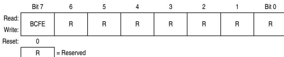
**Figure 17-8. Break Flag Control Register (BF CR)**
