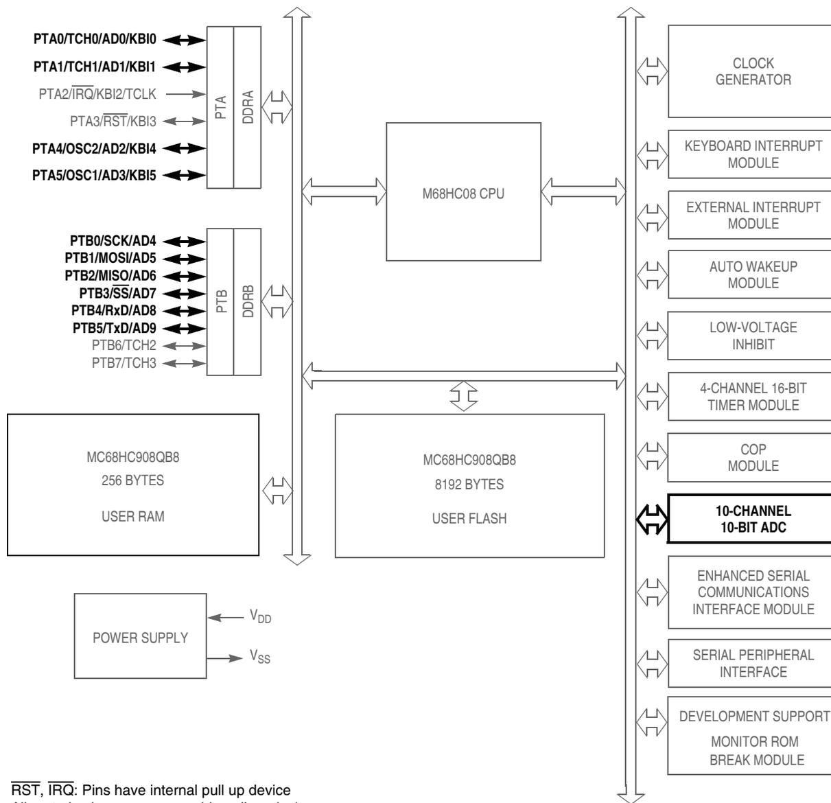
$\overline{RST}$ ,  $\overline{IRQ}$ : Pins have internal pull up device
