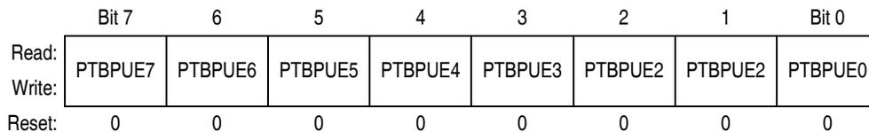
**Figure 12-8. Port B Input Pullup Enable Register (PTBPUE)**
