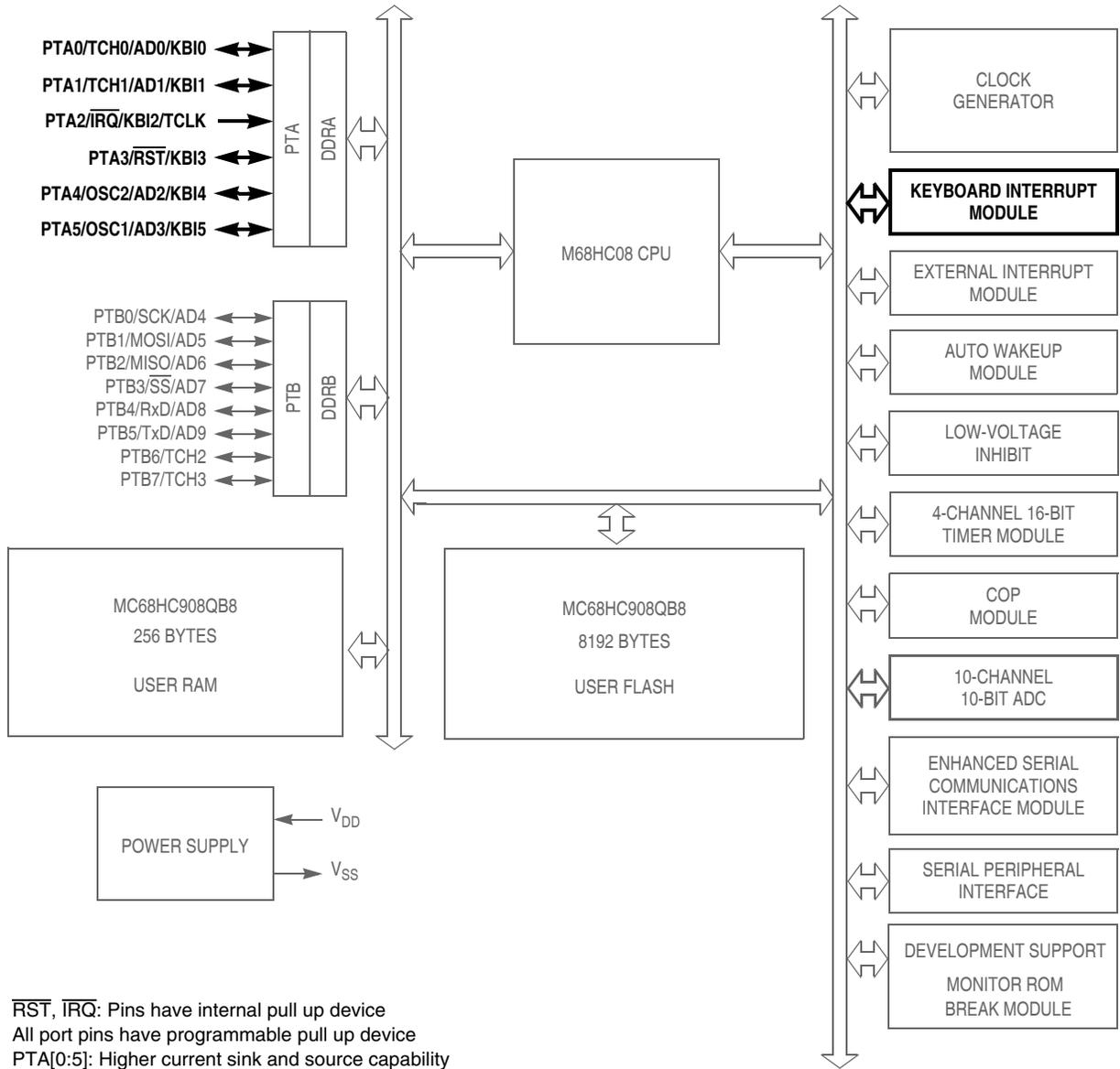
**Figure 9-1. Block Diagram Highlighting KBI Block and Pins**
