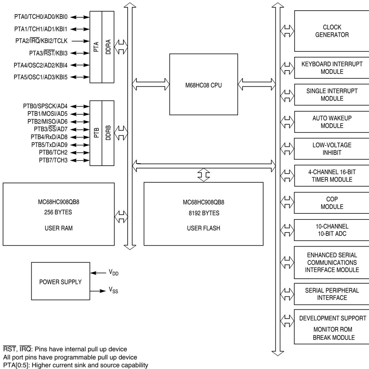
Figure 1-1. Block Diagram
