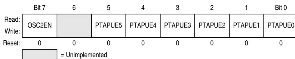
**Figure 12-4. Port A Input Pullup Enable Register (PTAPUE)**
