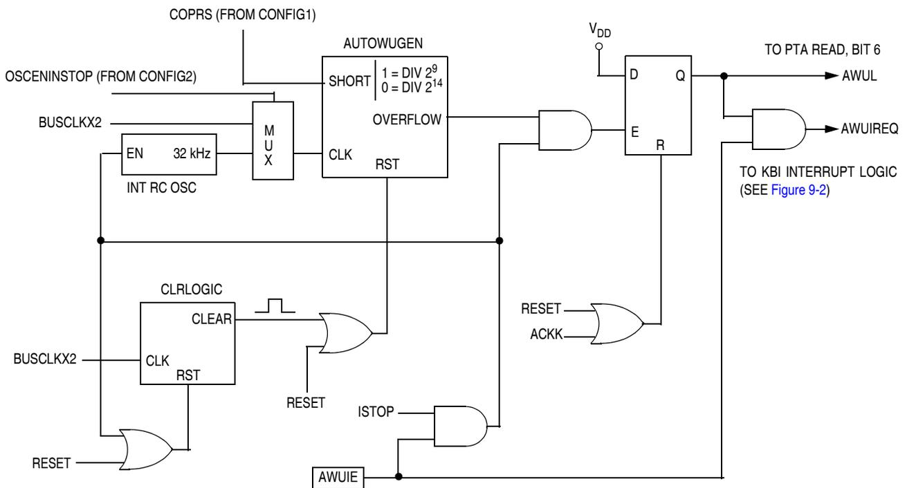
**Figure 4-1. Auto Wakeup Interrupt Request Generation Logic**
