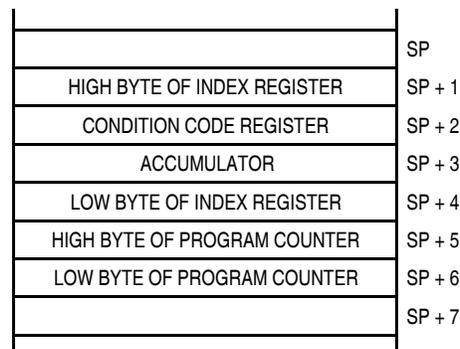
**Figure 17-17. Stack Pointer at Monitor Mode Entry**
