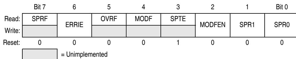
**Figure 15-14. SPI Status and Control Register (SPSCR)**
