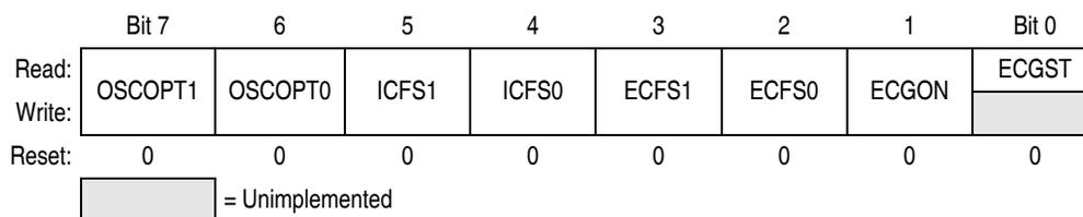
**Figure 11-4. Oscillator Status and Control Register (OSCSC)**
