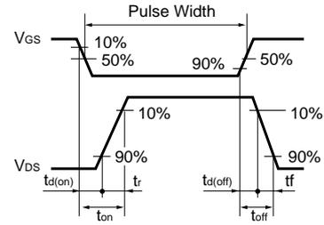
Fig.11 Switching Waveforms
