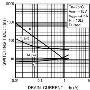
Fig.8 Switching Characteristics
