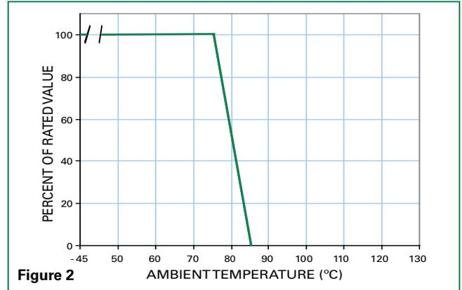
For applications exceeding 75°C ambient temperature, the peak surge current and energy ratings must be reduced as shown.
