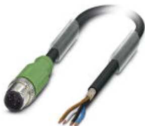
Sensor/actuator cable, 4-position, PUR halogen-free, black-gray RAL 7021, shielded, Plug straight M12, coding: A, on free cable end, cable length: 10 m
