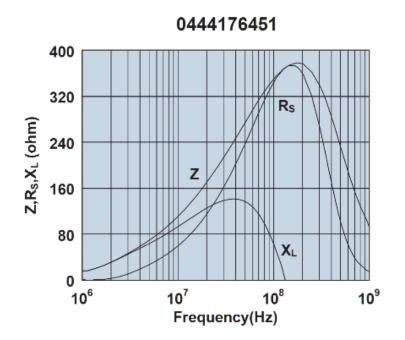
Impedance, reactance, and resistance vs. frequency.
