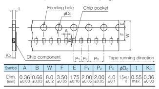
• Pitch 2 mm (Punched Carrier Taping): Size 0402
