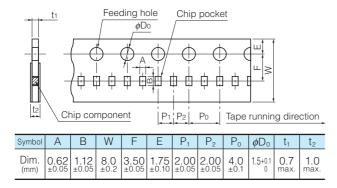
• Pitch 4 mm (Punched Carrier Taping): Size 0603
