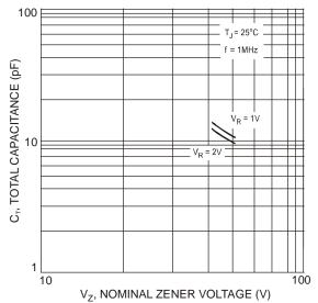
Fig. 6 Typical Total Capacitance vs. Nominal Zener Voltage
