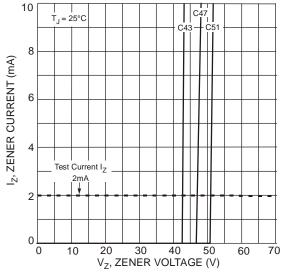
Fig. 4 Typical Zener Breakdown Characteristics
