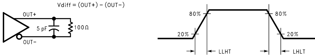
Figure 5. DS90CF563 (Transmitter) LVDS Output Load and Transition Times
