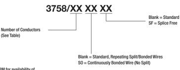
Note: Available in standard 275 ft rolls. Contact 3M for availability of additional conductor counts and/or custom roll lengths
