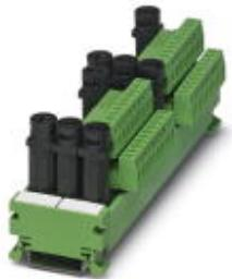
Fuse module, with screw connection, COMBICON connectors with stand-off and encoding against incorrect connection, for mounting on NS 35/7,5 or NS 32
