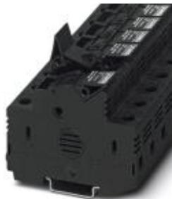
Fuse terminal block with light indicator, for cartridge fuse insert 10.3 x 38 mm, cross section: 1.5 - 25 mm<sup>2</sup>, AWG: 16 - 4, width: 18 mm, color: Black
