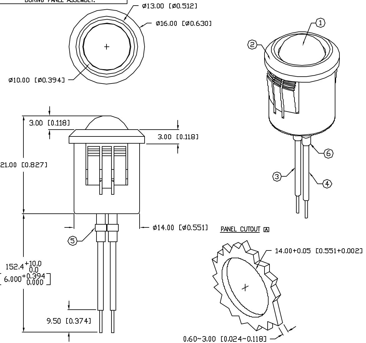
\*UNLESS OTHERWISE SPECIFIED TOLERANCES PER DECIMAL PRECISION ARE: X=±1 ( $\pm 0.039$ ), XX=±0.5 ( $\pm 0.020$ ), XXX=±0.25 ( $\pm 0.010$ ), XXXX=±0.127 ( $\pm 0.005$ ), LEAD SIZE=±0.05 ( $\pm 0.002$ ), LEAD LENGTH=±0.75 ( $\pm 0.030$ ), MIN=  $\pm 0.00$  DECIMAL PRECISION MAX.=  $\pm 0.00$  DECIMAL PRECISION
