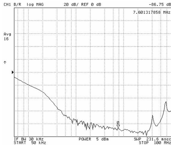
Figure 4 - Common Mode attenuation, 0.05-100 MHz. Source and load resistances are 50 Ω. Two 0.47 μF Y-caps to common line. Vertical scale: 20 dB/div, with zero dB level marked by arrow.
