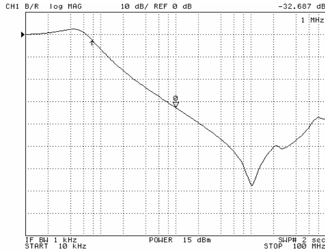
Figure 4 - F4810/F2410 - Common Mode attenuation, 0.2-100 MHz. Source and load resistances are 50 Ω. Two 0.1 uF Y- caps to common line. Vertical scale: 10 dB/div, with zero dB level marked by arrow.
