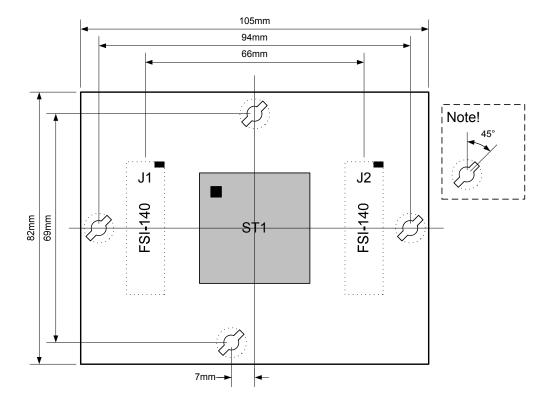
The board thickness should be 1.6mm to be compatible with the clips.
