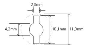
The board thickness should be 1.6mm to be compatible with the clips.
