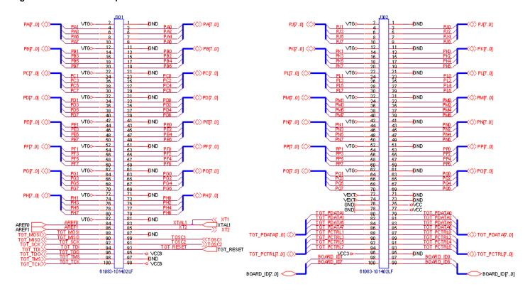
Table 3-2. STK600 J301 "expand0" connector pinout.
