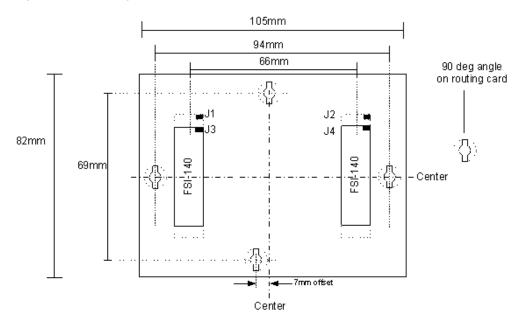
Figure 1-3. Clip hole dimensions.
