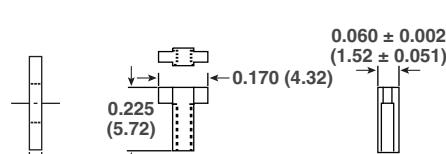
**On Contact Polarizing Key (Field Insertable)**
