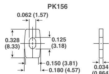
Between Contact Polarizing Key
