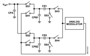
Figure 33. Equivalent Input Circuit
