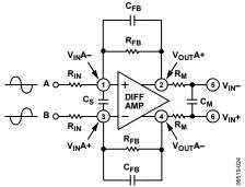
Figure 30. Differential Amplifier Configuration
