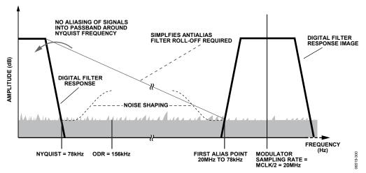
$Figure~28.~Antialias~Example~Using~the~AD7765~in~Normal~Mode, Decimate~128 \times~Using~MCLK/2 = ICLK = 20~MHz$
