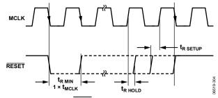
Figure 39. RESET Timing Synchronous to MCLK
