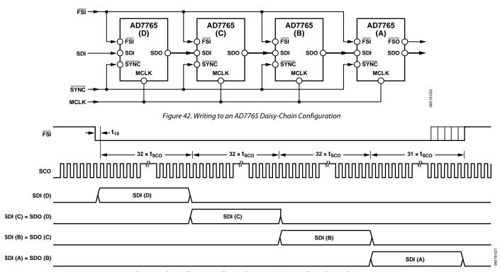
Figure 43. Daisy-Chain Write Timing Diagram; Writing to Four AD7765 Devices
