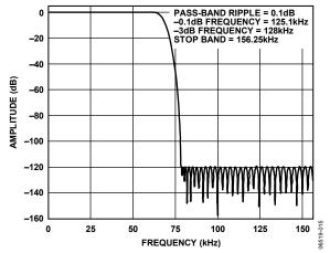
Figure 26. Filter Frequency Response
