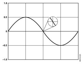
Figure 45. Maximum Slew Rate of the Same Frequency Sine Wave as in Figure 44 with an Amplitude of 1 V p-p
