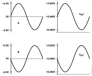
Figure 31. Differential Amplifier Signal Conditioning
