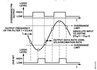
Figure 37. OVERRANGE Pin and OVR Bit vs. Absolute Voltage
