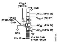
Figure 46. AD7765 Supply Decoupling
