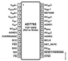
Figure 5. Pin Configuration
