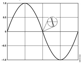
Figure 44. Maximum Slew Rate of a Sine Wave with an Amplitude of 2 V p-p
