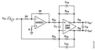
Figure 32. Single-Ended-to-Differential Conversion
