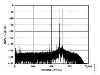
Figure 19. Normal Power Mode; IMD,  $f_{\rm IN}$  A = 49.7 kHz,  $f_{\rm IN}$  B = 50.3 kHz, 50 kHz Center Frequency, 128× Decimation Rate
