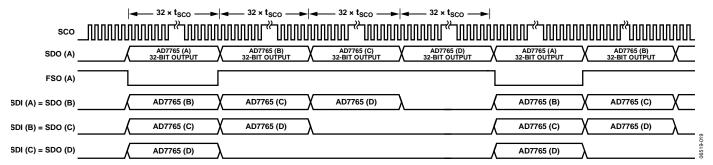
Figure 41. Daisy-Chain Mode, Data Read Timing Diagram (for the Daisy-Chain Configuration Shown in Figure 40)
