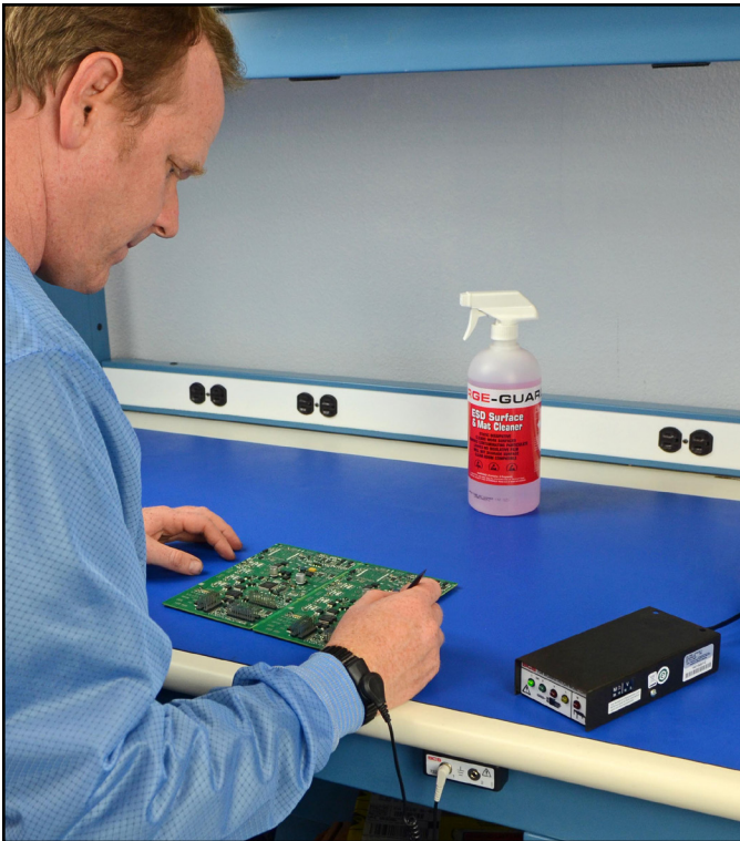
Figure 8. Using the 724 Workstation Monitor
