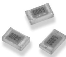
This tiny thin film chip is manufactured by sputtering pure metals onto a high purity alumina base. This process ensures the element remains stable in performance over a long life. The LT73 is equally suited to temperature compensation or thermal protection when incorporated within the appropriate electronics. This range of sensors are finished in a tough epoxy seal and are available on tape for high speed auto placement.
