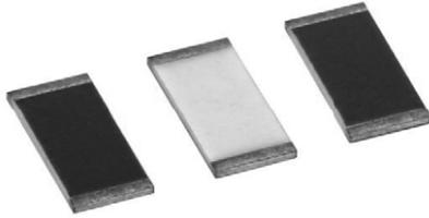
These chip resistors are available in wraparound terminations styles in 8 case sizes. They incorporate self passivated enhanced tantalum nitride resistor film to give superior performance on moisture resistance, electrostatic discharge, voltage coefficient, power handling and resistance stability. The terminations consist of an adhesion layer, a leach resistant nickel barrier, and solder coating (lead (Pb)-free). This product will out-perform all requirements of AEC-Q200.
