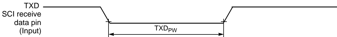
Figure 10-17 TXD Pulse Width
