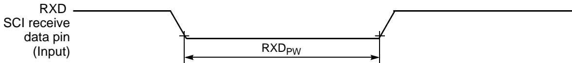
Figure 10-16 RXD Pulse Width
