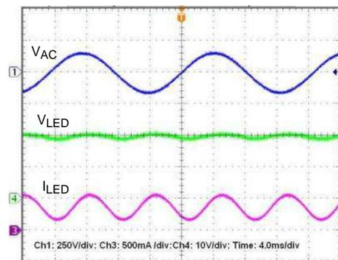
Figure 17. Output Current and Voltage Waveforms (120VAC)
