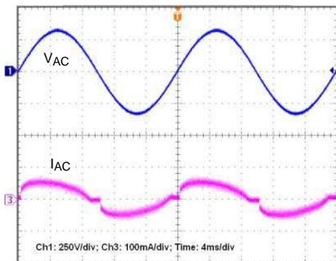
**Figure 12. Input Voltage and Input Current (230VAC)**
