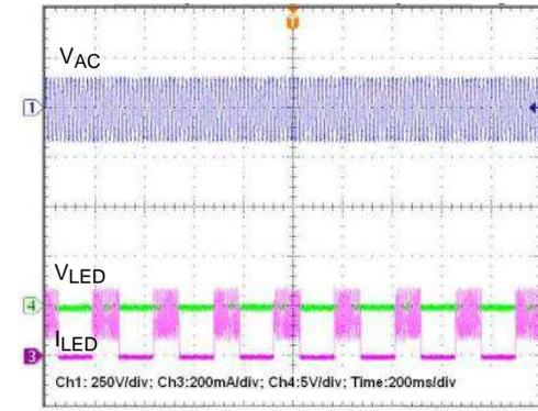
Figure 19. Output Short Circuit Waveforms (120VAC)
