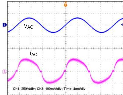
**Figure 13. Input Voltage and Input Current (120VAC)**
