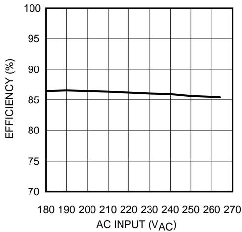
Figure 4. Efficiency vs AC Input
