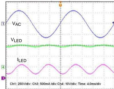
Figure 16. Output Current and Voltage Waveforms (230VAC)
