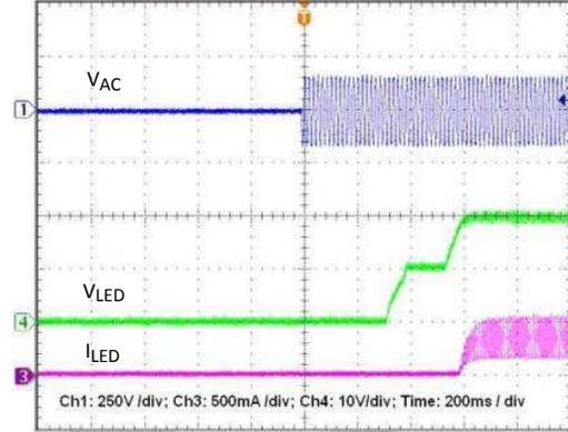
Figure 15. Power Up Output Voltage and Current (120VAC)
