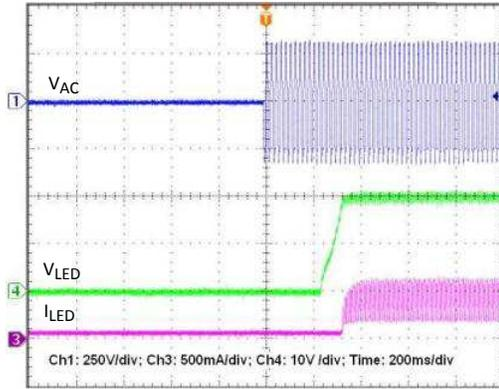
Figure 14. Power Up Output Voltage and Current (230VAC)
