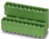
Header, Nominal current: 10 A, Rated voltage (III/2): 320 V, Number of positions: 3, Pitch: 5 mm, Color: green, Contact surface: Tin, Mounting: Soldering, The article can be aligned to create different nos. of positions! In combination with MVSTB or FKCV plug components, both an MVSTBW (or FKCVW) and an MVSTBR plug (or FKCVR) must be used. Combination with TMSTBP plug components is not possible!
