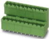
Header, Nominal current: 10 A, Rated voltage (III/2): 320 V, Number of positions: 3, Pitch: 5 mm, Color: green, Contact surface: Tin, Mounting: Soldering, The article can be aligned to create different nos. of positions! In combination with MVSTB or FKCV plug components, both an MVSTBW (or FKCVW) and an MVSTBR plug (or FKCVR) must be used. Combination with TMSTBP plug components is not possible!
