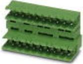
Header, Nominal current: 10 A, Rated voltage (III/2): 320 V, Number of positions: 3, Pitch: 5 mm, Color: green, Contact surface: Tin, Mounting: Wave soldering, Can be aligned! Mounting flange: Order no. 1736771, 1736768. In combination with MVSTB or FKCV plugs, both an MVSTBW (or FKCVW) and an MVSTBR plug (or FKCVR) must be used. Combination with TMSTBP plugs is not possible!
