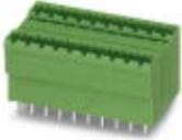
Header, Nominal current: 10 A, Rated voltage (III/2): 320 V, Number of positions: 3, Pitch: 5 mm, Color: green, Contact surface: Tin, Mounting: Wave soldering, In combination with MVSTB or FKCV plug components, both an MVSTBW (or FKCVW) and an MVSTBR plug (or FKCVR) must be used. Combination with TMSTBP plug components is not possible!
