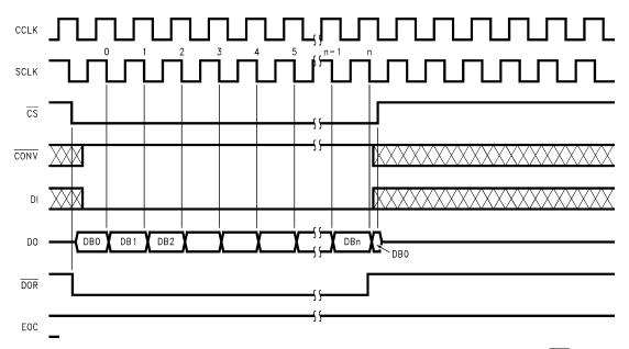
Figure 49. ADC12038 Read Data without Starting a Conversion Using CS
