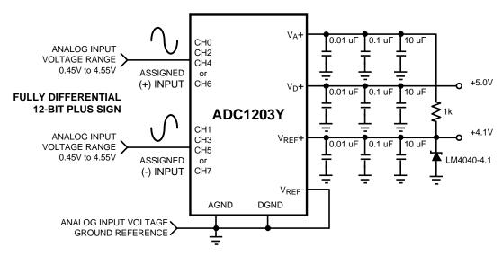
Figure 69. Fully Differential Biasing
