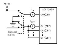
Figure 42. Leakage Current
