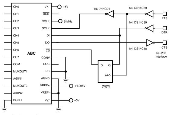
**Note:**  $V_A^+$ ,  $V_D^+$ , and  $V_{REF}^+$  on the ADC12038 each have 0.01  $\mu F$  and 0.1  $\mu F$  chip caps, and 10  $\mu F$  tantalum caps. All logic devices are bypassed with 0.1  $\mu F$  caps.
