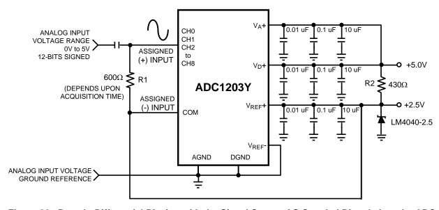
Figure 66. Pseudo-Differential Biasing with the Signal Source AC Coupled Directly into the ADC
