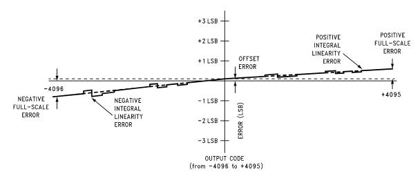
Figure 7. Simplified Error Curve vs. Output Code after Auto Calibration Cycle
