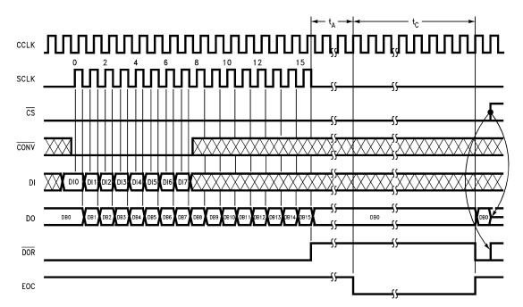
Figure 54. ADC12038 Conversion with CS Continuously Low and 16-Bit Digital Output Format
