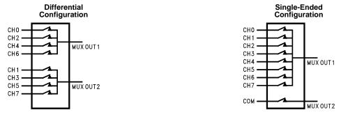
A/DIN1 and A/DIN2 can be assigned as the + or - input
