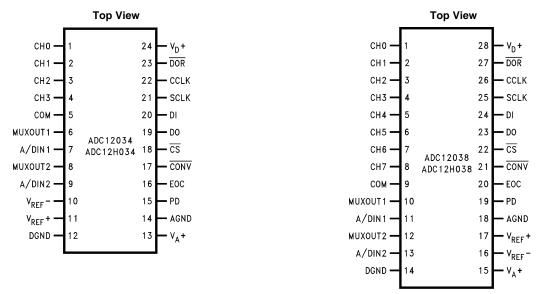
Figure 3. 24-Pin Wide Body SOIC, PDIP, SSOP Packages See Package Numbers DW0024B, NAM0024D, DB0024A
