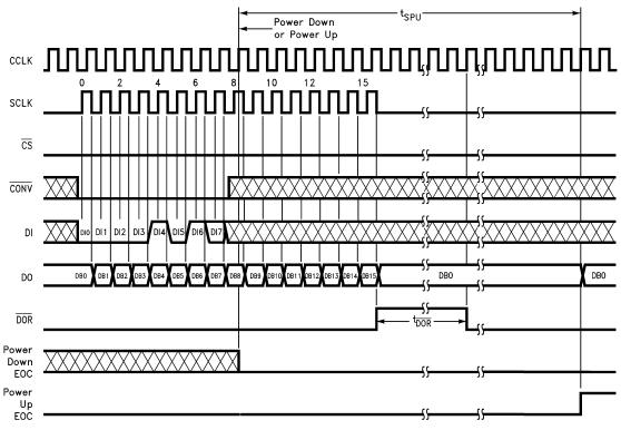
Figure 56. ADC12038 Software Power Up/Down with CS Continuously Low and 16-Bit Digital Output Format
