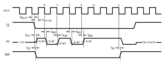
Figure 46. DO Data Output Timing Using CS
