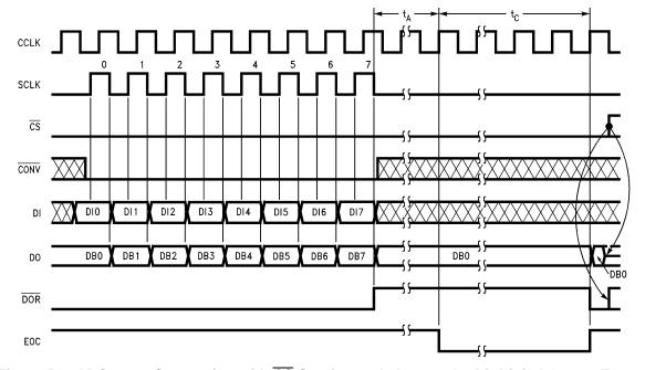
Figure 53. ADC12038 Conversion with CS Continuously Low and 8-Bit Digital Output Format
