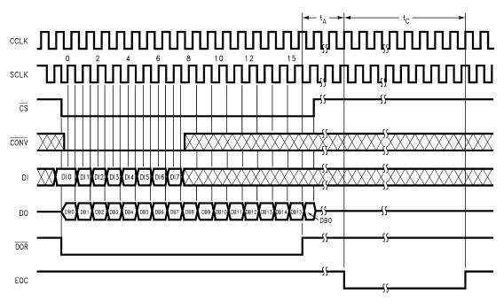
Figure 52. ADC12038 Conversion Using CS with 16-Bit Digital Output Format
