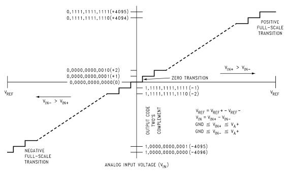
Figure 5. Transfer Characteristic
