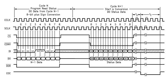
**Note:** In order for all 9 bits of Status Information to be accessible, the last conversion programmed before Cycle N needs to have a resolution of 8 bits plus sign, 12 bits, 12 bits plus sign, or greater.
