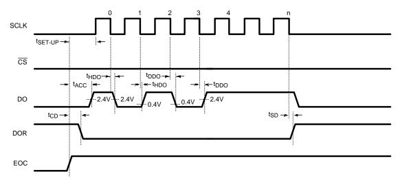
Figure 47. DO Data Output Timing with CS Continuously Low
