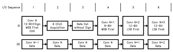
Figure 62. Changing the ADC's Conversion Configuration
