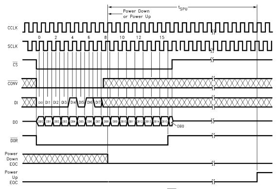
Figure 55. ADC12038 Software Power Up/Down Using CS with 16-Bit Digital Output Format
