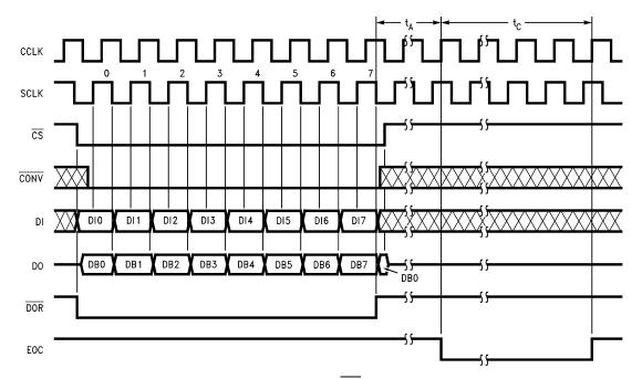
Figure 51. ADC12038 Conversion Using CS with 8-Bit Digital Output Format
