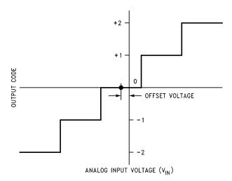
Figure 8. Offset or Zero Error Voltage
