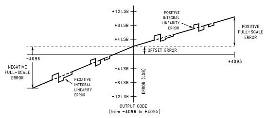
Figure 6. Simplified Error Curve vs. Output Code without Auto Calibration or Auto Zero Cycles
