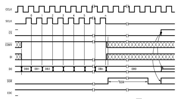
Figure 50. ADC12038 Read Data without Starting a Conversion with CS Continuously Low
