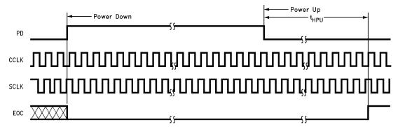
**Note:** Hardware power up/down may occur at any time. If PD is high while a conversion is in progress that conversion will be corrupted and erroneous data will be stored in the output shift register.
