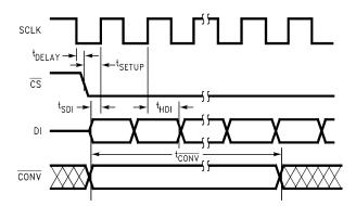
Figure 45. DI Data Input Timing
