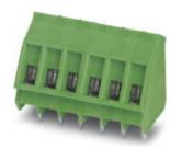
PCB terminal block, Nominal current: 24 A, Nom. voltage: 400 V, Pitch: 5.08 mm, Number of positions: 3, Connection method: Screw connection with tension sleeve, Mounting: Wave soldering, Conductor/PCB connection direction: 55 °, Color: green, The article can be aligned to create different nos. of positions!
