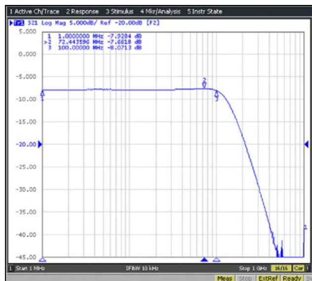
FIGURE 13. AMPLIFIER FREQUENCY RESPONSE AT 200MSPS
