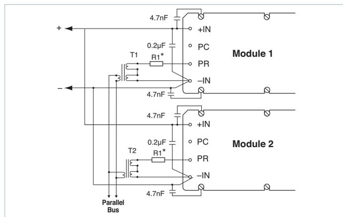
Figure 10 — Transformer-coupled interface
